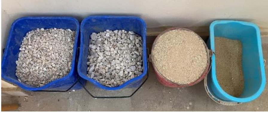
Fig. 2. Coarse and Fine Aggregate Fractions Obtained from Sieve Analysis
