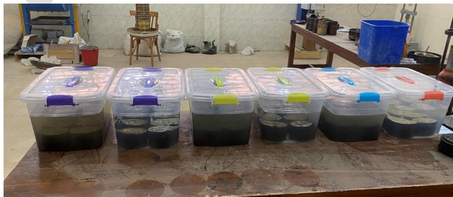
Fig.3. Moisture Conditioning of Specimens Under Freshwater and Sewage Water
